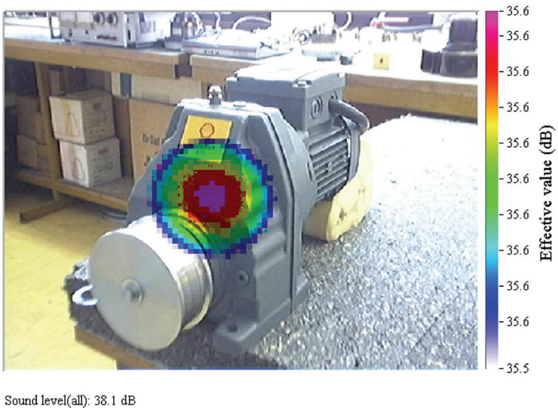
Fig. 7. An acoustic image with noise source of a gear unit with a crack in the tooth root
