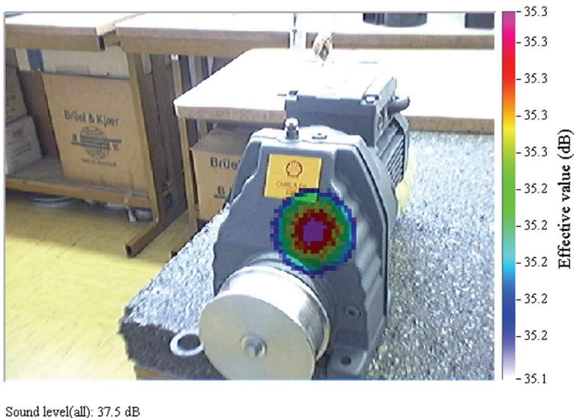
Fig. 5. An acoustic image with noise source of a gear unit of a faultless gear
