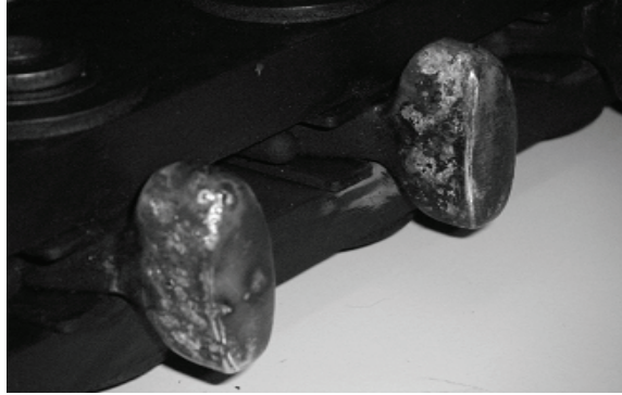
Fig. 5. Tap selector fixed contacts damaged by arcing
